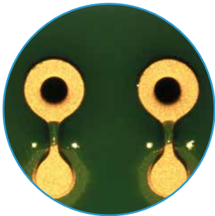
Solder mask edge printing No bleeding
