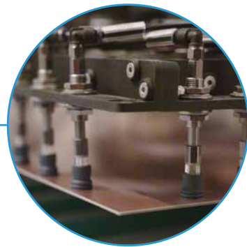
The gripper can be adjusted to different substrate sizes
