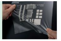
Sensors: Integration of RFID tags and other electronic components into formerly "idle" parts, such as load floors and steering wheels
