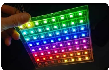
In-mould display with RGB LED's
