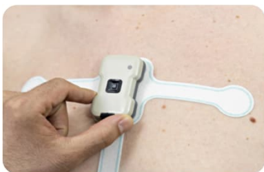
ECG smart patch with external reader and magnetic snap connectors
